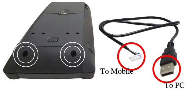
1: Unscrew the screws (2) on the back cover of the Hand Held Computer to access the Connector Slot.
