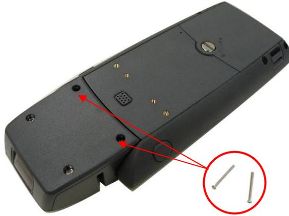
4: To use the attached screws (2) to fix the 2-in-1 MSR module to the Hand Held Computer.
