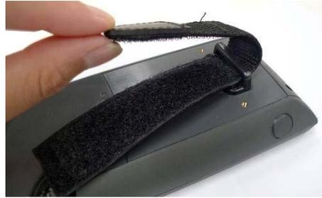
1: Fasten the Hand Strap Plastic Ring with the screws (2) to the screw holes at rear side of the system.
