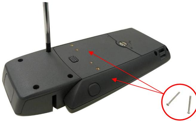
5: Use the attached screws (2) to fix the MSR module to the Hand Held Computer as above photo shows.
