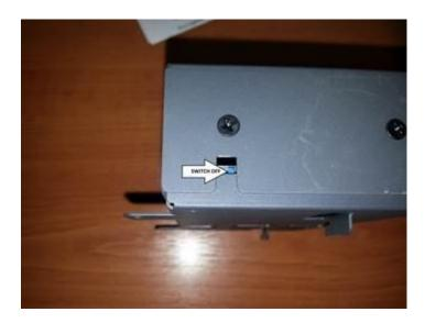
When ready to use move the Battery protect switch on as per photo below.
