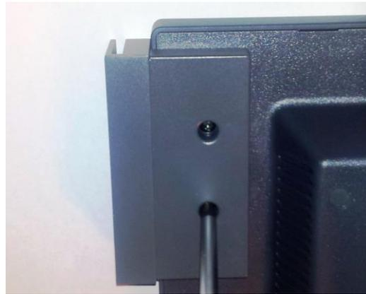
The RFID card can be read either by just getting the card with in one or two cm of the reader or can be slide into the MSR slot allowing the MSR reader to act as a clip to hold the MSR in place as shown below.
