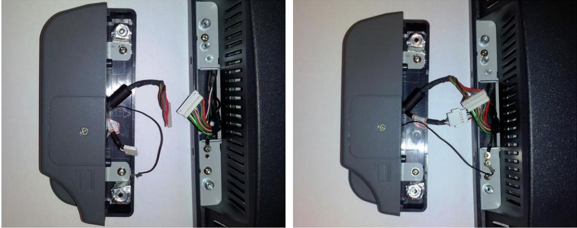
Now using the two screws provided attach the RFID/MSR to the unit.
