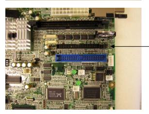
Locate the 4 pin jumper J4 [to the right of the black IDE1 connector] and remove both jumpers to enable the I-Button.
