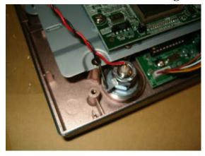
Remove the two front bezel attaching screws located towards the bottom of the back of the unit head.
