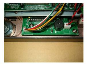
Mount the I-Button circuit board to the front bezel and fit the connectors as shown.
