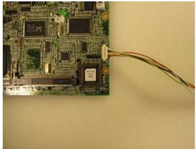
Fit the I-Button cable connector to the main board as shown
