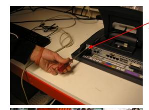
Slacken the two holding screws & slide the main board out of the unit.
