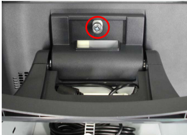
a. Loosen the thumbscrew (1)
