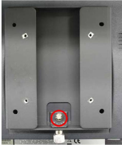
Install screw to secure thumbscrew clip
