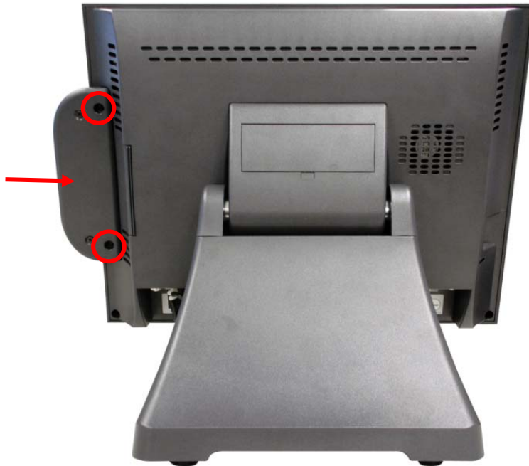
c. Slide the MSR into the position and tighten the screw to finish the installation. Be careful not to pitch the cable when installing.
