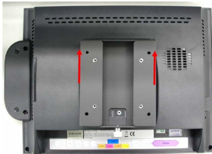
Install screw to secure thumbscrew clip
