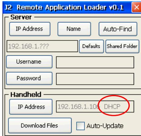
It is highly recommend that the IP address for the handheld use a fixed IP address. A fixed IP address is needed for quick reconnection to the network when the wireless signal is lost or when using auto-roaming. If *Auto-Find* is used it will automatic change the DHCP IP address of the handheld to a fixed IP address.
