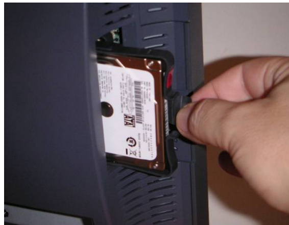
HDD slide in-slide out drive bay
