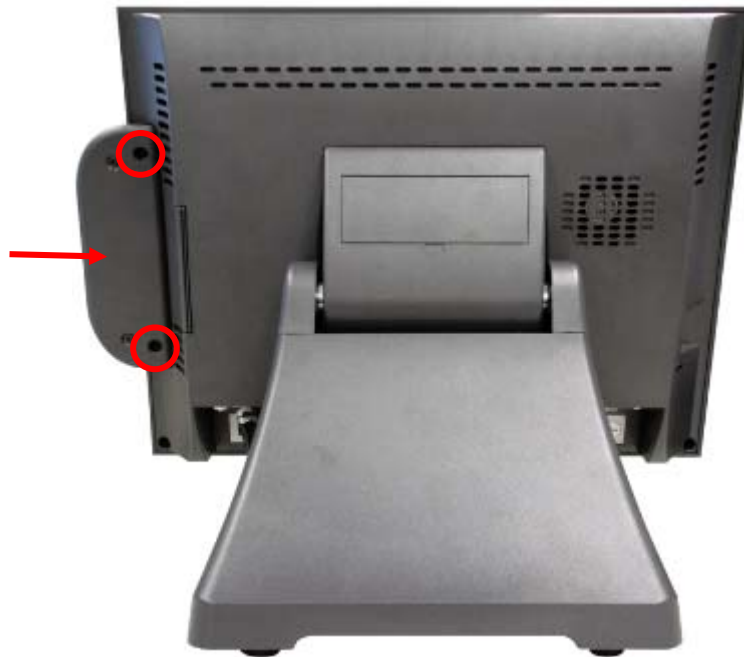
c. Slide the MSR into the position and tighten the screws to finish the installation. Be careful not to pitch the cable when installing.
