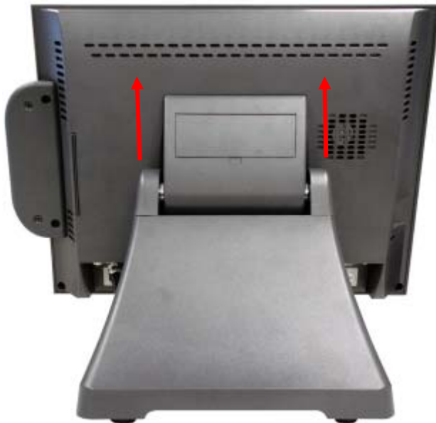
b. Lift the panel up and separate it from the stand bracket
