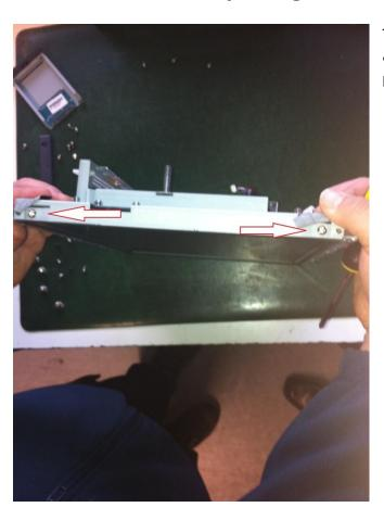
Turn the LCD over, pull back the black tape & remove the two screws as shown in the photo.
