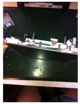
Place the LCD on its edge & remove the two screws as shown in the photo
