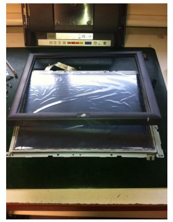
Turn the unit over & lift off the bezel.
