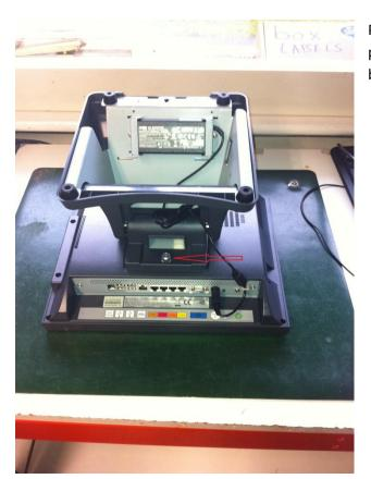
Place the unit screen side down on a protective mat. Undo the screw securing the base & remove the base.
