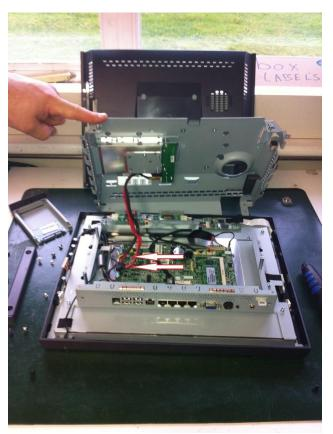
Uplug the SATA cables & remove the metal panel.
