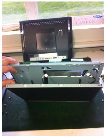
Pull the LCD out of its mounting panel.
