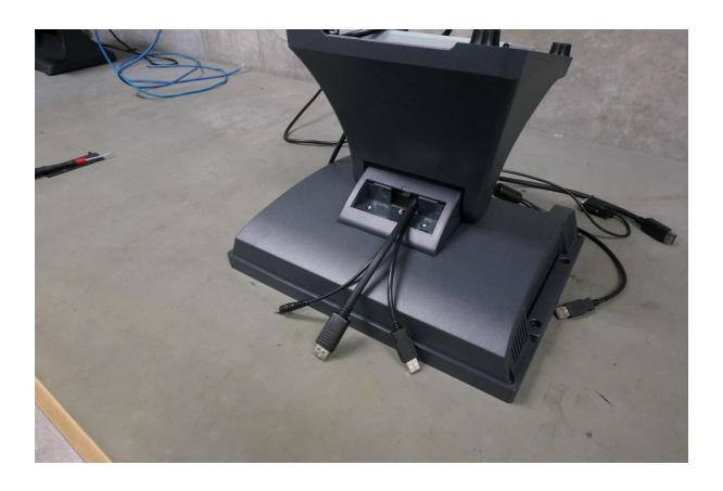
Step 6. Attached cables to 14" LED Display
