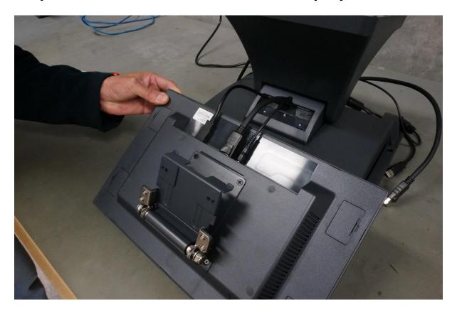
Step 6. Fit Display to mounting position on J2 680
