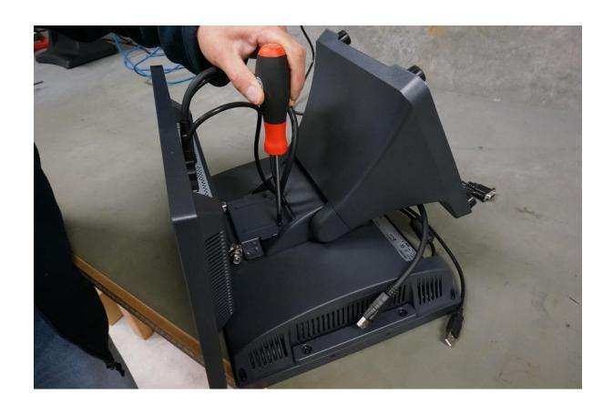
**Step 7. Secure cables to ports**
