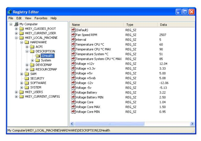
Register keys that are followed with the letters *MAX* or *MIN* are the J2 recommend maximum or minimum value for the register key with the same name. Some values may only have a maximum or minimum value like *Voltage Battery* of *Temperature CPU* as the other extreme has no relevant meaning.
