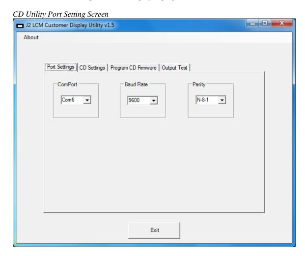
Set the *ComPort*, *Baud Rate* and *Parity* to match the current setting of the customer display. Once this is done the setting of the display may be changed.
