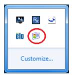
By right clicking of the icon a few options are available. The allow for the iButton to output the serial number data as track 1&2 MSR data, track 1 data or track 2 data. There is also an option to stop the emulator for trouble shooting purposes. The Track selection will be stored in the system registry and retain after a reboot.
