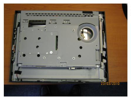
Remove the 10 screws holding the metal cover in & remove the cover.
