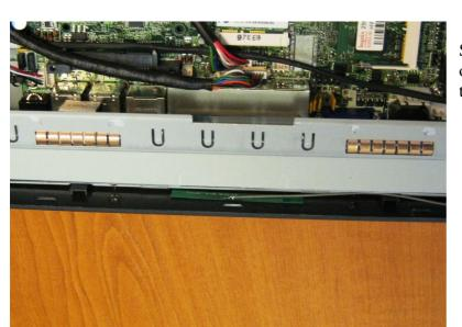
Guide the antennae cables through the gap in the corner of the metal cage as shown in the photo.
