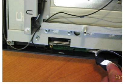
Stick the other antenna underneath the touchscreen cable on the side of the unit.
